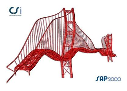
Today, things are different – the structural engineer generates 3-D mathematical structural models in the computer, straight from initial design drawings produced by an architect, designer or artist. The engineer then uses software to subject these models to simulated earthquakes or blowing winds. The software produces 3-D animations that graphically depict the swaying and stress variations under the influence of the loads.
